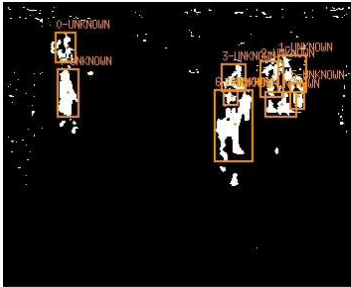
Figure 2.1 Bounding boxes, representing moving regions, that were found by the motion detector algorithm
