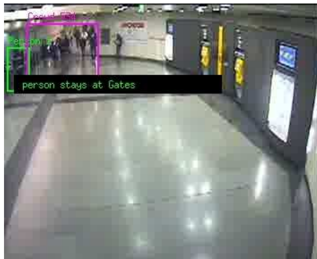
Figure 2.5 Person detected staying at the gates (smaller bounding box) and a crowd.
