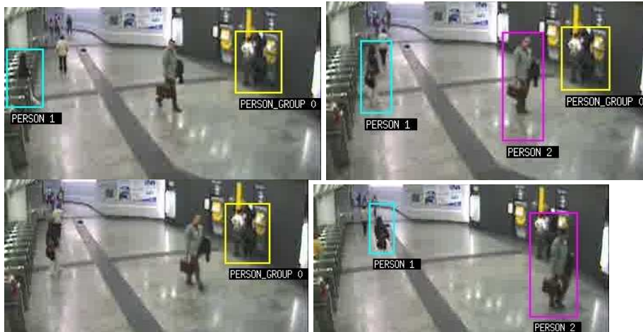
Fig. 2. Tracked objects in the Torino underground station ‘Diciotto Dicembre’. Images corresponding to a video sequence acquired at 25 fps.
