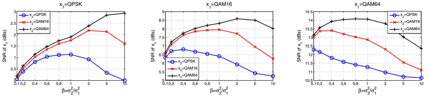
Fig. 3. For each value of  $\beta$ , SNR of  $x_1$  is optimized to achieve target FER of  $10^{-2}$ . 3GPP punctured rate 1/2 turbo code is used with 5 decoding iterations while the frame length of  $x_1$  is fixed to 1056 information bits.
