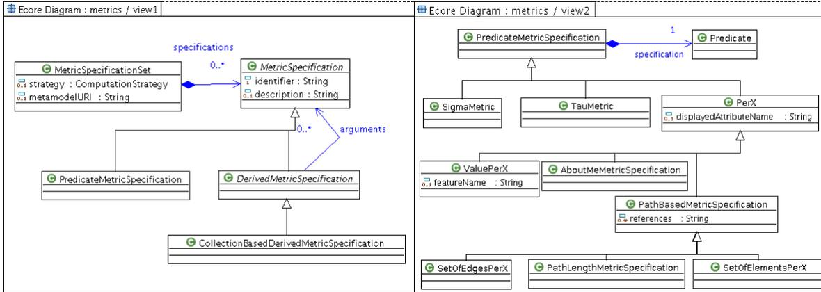
Figure 3: The core of the metric specification metamodel
