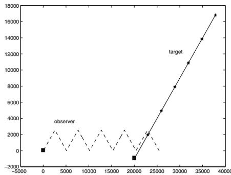
Fig. 1. Simulation scenario. Total observation time 1 hour, sampling interval 4s. Initial relative distance 20025m, target speed 7m/s, observer speed 10m/s. Trajectories: target (plain line), maneuvering observer (dashed line), initial positions (black squares).
