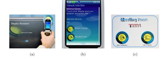
Fig. 7: The user interface for the manual method: user interacting with a display service (a), the mobile phone user interface (b) (shows that two services are selected) and the control panel for the remote services (c).
