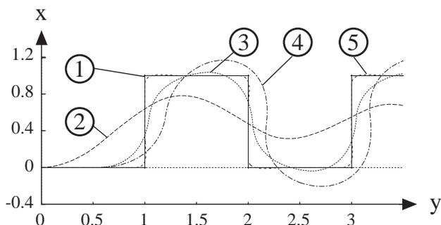
This figure shows various motions for a trajectory physically impossible (curve 1). Changing the base distance (curves 2 and 5) enables to choose how much we want to smooth the trajectory. Changing  $\alpha$  within a certain range, and with the same  $B$  affects only the speed of the motion. Changing  $B$  (curves 2, 3 and 4) affects the damping of motion.
