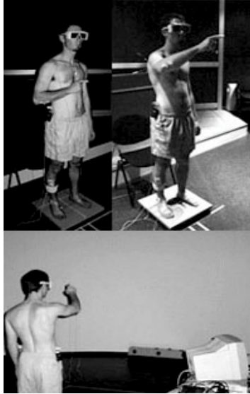
Fig. 1. Installation of the subject in the VE-room. Subject stood on the forceplate and executed pointing movements from the starting position toward the virtual target. The Optotrack system is placed at the bottom of the curved-screen.
