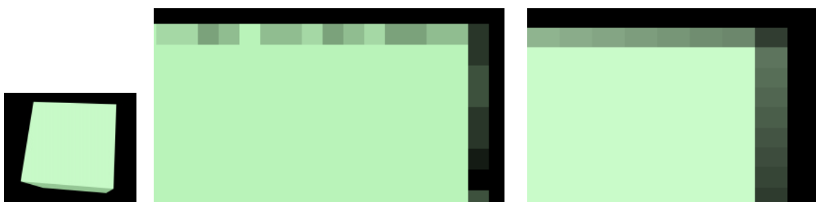
Figure 14: antialiasing of a cube (left), obtained with the ray tracing software Pov Ray (centre) and with a visibility map (right). The antialias threshold value used with POV is the value recommended in its documentation.
