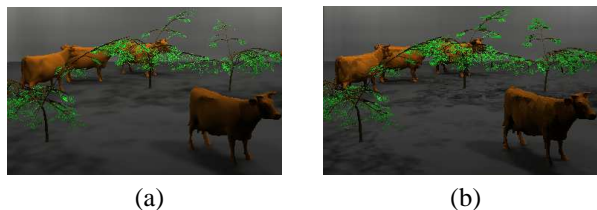
Figure 10: Scene containing 43,000 polygons. (a) the original image and (b) the image generated with cluster reduction.
