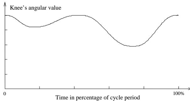
Figure 2: Approximation of the knee angle trajectory by 5-degree polynomial.
