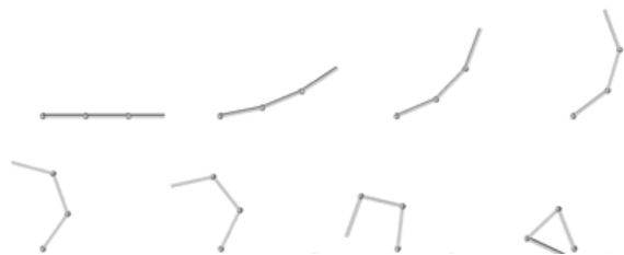
Figure 7: A hierarchy of motions. Each joint of the articulated arm just defines rotation in its parent referential.
