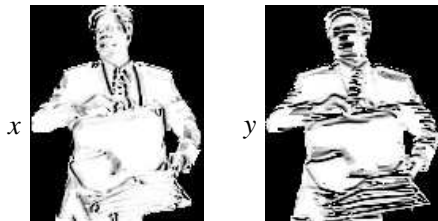
Figure 5: Example of discontinuity maps. Dark regions represent potential surface discontinuities.
