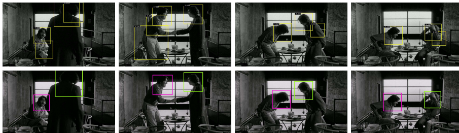
Fig. 2. Upper body detections (top row) and tracks (bottom row) after classification post-processing for a sample test sequence of C&C . The bounding box colours indicate different tracks. Note the improvement due to the tracking where false positives have been removed, as well as the high accuracy despite motion, articulations and self-occlusions.
