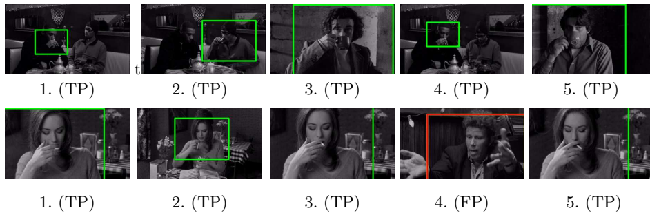
Fig. 6. The five highest ranked drinking (top) and smoking (bottom) detections on CC . For drinking the first false positive (FP) is ranked 11th.
