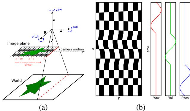
**Fig. 1.** (a) Pushbroom acquisition principle: the camera is moving straight along the  $x$  axis and recording 1-D images over time denoted by  $n$ ;  $y$  is the camera axis and  $z$  the orthogonal axis to the image plane. We define the orientation of the camera with the yaw (rotation about  $z$ ), the roll (rotation about  $x$ ) and the pitch (rotation about  $y$ ). (b) Example of warps in a regular checkerboard when the pushbroom camera is tilting around its 3 rotation axes.
