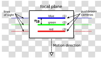
**Fig. 2.** Focal plane geometry of an observation satellite with 3 pushbroom cameras: blue, green and red (respectively 1,2 and 3). What is seen by the camera 2 at time  $n$  will be seen by the camera 1 at time  $n + \tau_{12}$  in the absence of attitude variations.
