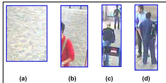
Fig. 3. (a) object is not present in the blob (object area = 0%); (b) object is partially present in the blob (object area = 50%); (c) and (d) object is totally present in the blob (object area = 100%).
