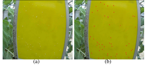
Figure 4. (a) A video-frame ; (b) Extraction of the insect locations in it.
