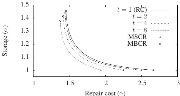
Figure 11. Optimal tradeoffs between storage and repair costs for  $k = 16$  and  $d = 24$ . Regenerating codes (RC) [10] are depicted as  $t = 1$ . For each  $t$ , both MSCR and MBCR are shown. Costs are normalized by  $\mathcal{M}/k$ .
