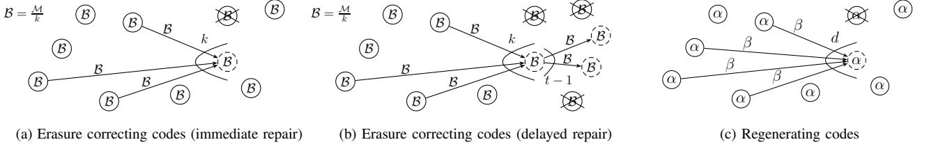
Figure 1. Repairing failures with codes. In a  $n$  device network, failed devices are replaced by new ones. The new devices get a given amount of data from live devices to repair the redundancy. In our examples,  $k = 3$ ,  $d = 4$ ,  $\mathcal{B} = 1$ ,  $\alpha = 1$ , and  $\beta = 1/2$ . Some example of gains for  $k = 32$  are given in Table I
