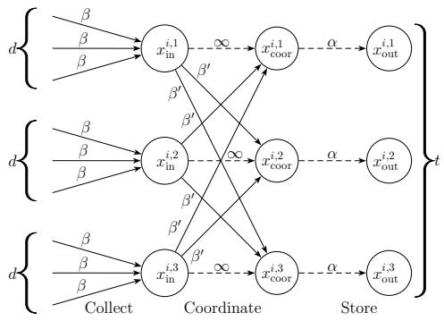
Figure 7. Information flow graph of a repair of  $t = 3$  devices. The internal nodes of the graph represent intermediary steps in the repair. First, each device collects  $\beta$  from  $d$  live devices. Second, devices coordinate by exchanging  $\beta'$  with each other. Third, they store  $\alpha$ . Plain edges correspond to network communication and dashed edges correspond to local communication.
