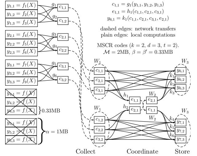
Figure 6. Coordinated regenerating codes based on linear codes. The system stores a file  $X$  and is compound of 5 devices. Device  $i$  stores 3 sub-blocks  $\{y_{i,1}, y_{i,2}, y_{i,3}\}$ . Devices 4 and 5 fail and are replaced by devices 6 and 7.
