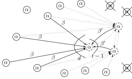
Figure 5. Repairing failures in coordinated regenerating codes. In a network of  $n$  devices storing  $\alpha$  bits, when  $t$  devices have failed,  $t$  new devices collect  $\beta$  bits from  $d$  live devices. They coordinate by exchanging  $(t-1)\beta'$  bits with other new devices and store  $\alpha$  bits.
