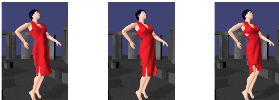
Figure 5: Example of stochastic collision detection and response in a cloth simulation (avatar 25000 faces, shirt 4400 faces, trousers 4000 faces).
