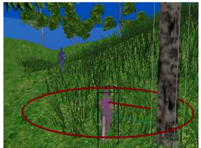
Figure 5. Simulated perception of the characters. The red circle represents the sensor-range, and the red line segment show the nearest obstacle.
