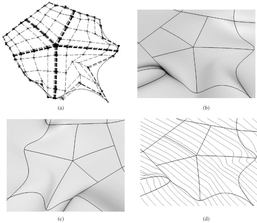
Fig. 11. (a) Control points of the pentagonal hole for  $\varepsilon = 0.1^\circ$ ; (b) the pentagonal hole and its adjacent surfaces when  $\varepsilon = 0.1^\circ$ ; (c) another view of surfaces in (b); (d) highlight lines of NURBS surfaces in (b).
