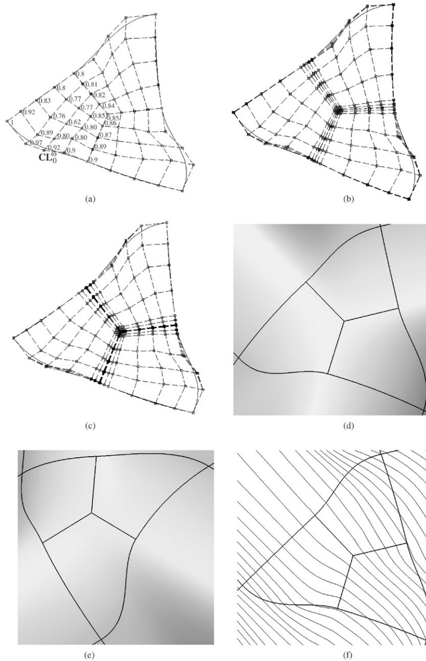
Fig. 10. Control points of the trigonal hole for (a)  $\varepsilon = 10^\circ$ , (b)  $\varepsilon = 1^\circ$ , (c)  $\varepsilon = 0.1^\circ$ ; (d) the trigonal patch and its adjacent surfaces when  $\varepsilon = 1^\circ$ ; (e) another view of surfaces in (d); (f) highlight lines of NURBS surfaces in (d).
