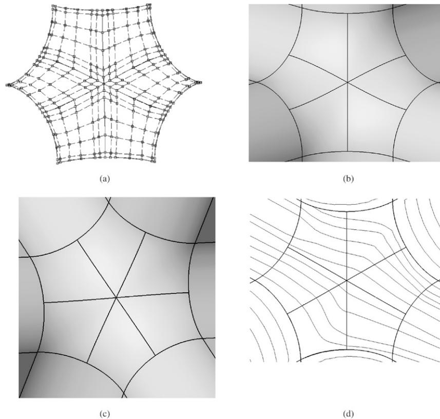
Fig. 12. (a) Control points of hexagonal hole for  $\epsilon = 1^\circ$ ; (b) the hexagonal hole and its adjacent surfaces when  $\epsilon = 1^\circ$ ; (c) another view of surfaces in (b); (d) highlight lines of NURBS surfaces in (b).
