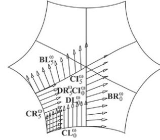
Fig. 8. Boundaries and cross-boundary derivatives of one patch.
