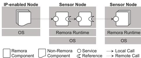
**Figure 3: Architecture of the Remora distribution model.**
