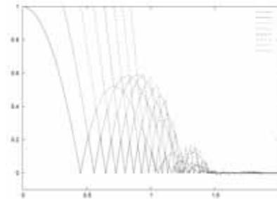
**Figure 9:** Vertical displacement of beads according to time
