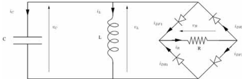
Figure 5: Electrical oscillator with 4 diodes bridge full-wave rectifier
