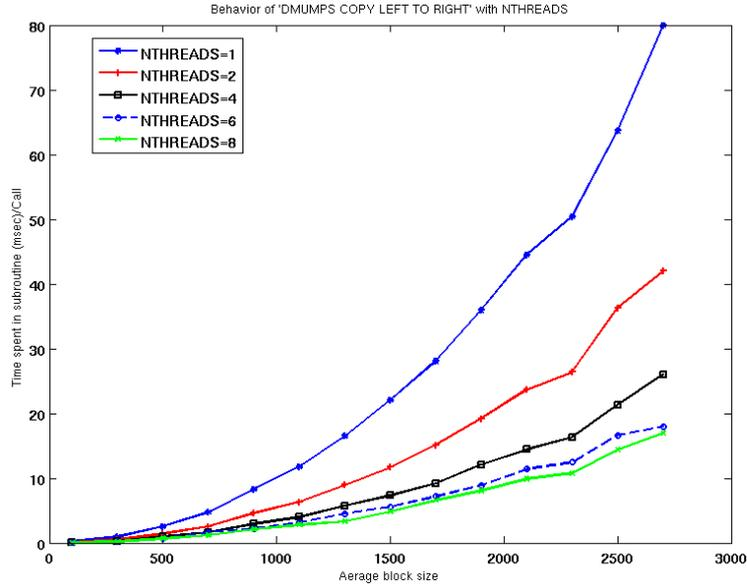
Figure 4: Behaviour of copyCB as a function of the number of threads. Each point on the x-axis refers to an interval of width 200. Testcase *DIMES*, Opteron.
