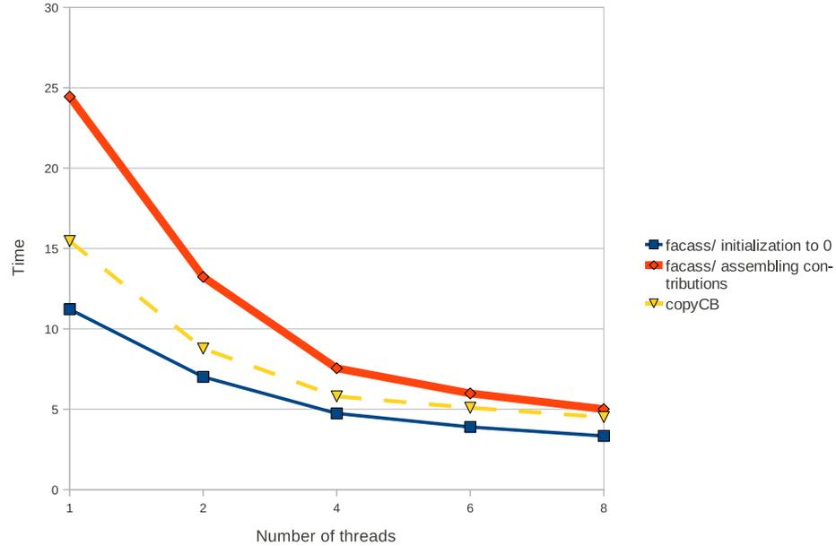
Figure 3: Assembly time as a function of the number of threads (testcase *AMAT30*), Opteron. The figure shows separately initialization to 0 and assembly of contributions blocks (both are part of the assembly routine *facass*). Time for copying contribution blocks (*copyCB*) is also given for comparison.
