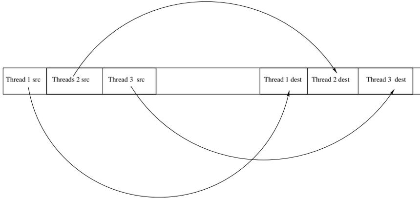
Figure 6: Working areas of threads during CopyCB Operations.
