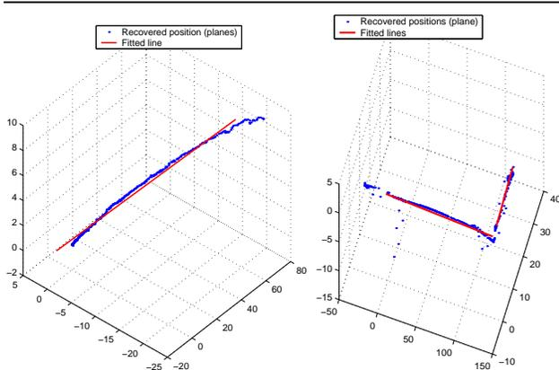
**Figure 4. Recovered positions (in 3D space) for the straight line trajectory (left) and the 2 perpendicular lines trajectory (left). The red line are the fitted 3D lines to each line segment.**
