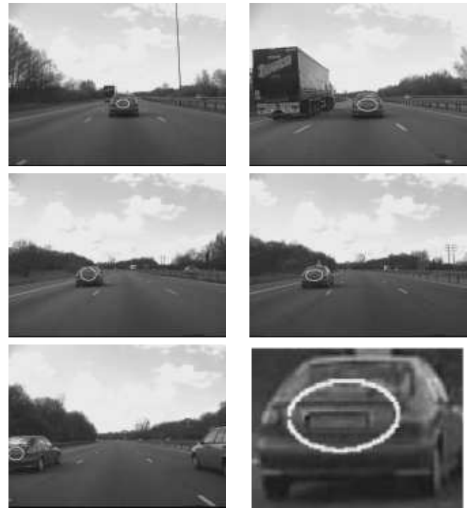
Figure 5: License plate tracking results: images 1, 187, 347, 417, 520 of the sequence, and a zoom made on image 417.
