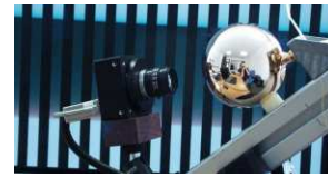
Figure 7: Catadioptric camera built from a Basler A201bc camera with a Fujinon 12.5 mm lens pointed at a roughly spherical mirror.
