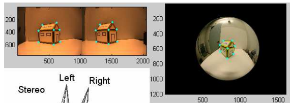
Figure 5: Combination of a pinhole and a fisheye camera. Top: input images and matching points. Bottom: estimated relative pose and 3D model.
