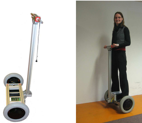
Fig. 6. The ChessWay personal transporter
