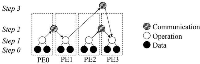
Fig. 5. Parallel reduction computation using four processing elements
