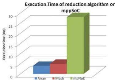
Fig. 6. Execution time on different mppSoC configurations
