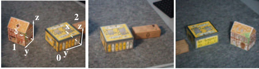
Figure 3: Images and parallelepipeds used for calibration.
