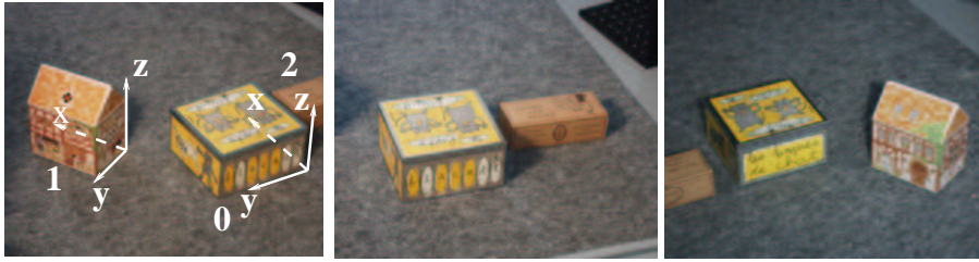
Figure 3: Images and parallelepipeds used for calibration.
