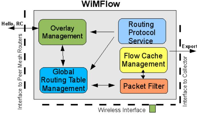
Fig. 4: Design of WiMFlow on a mesh router
