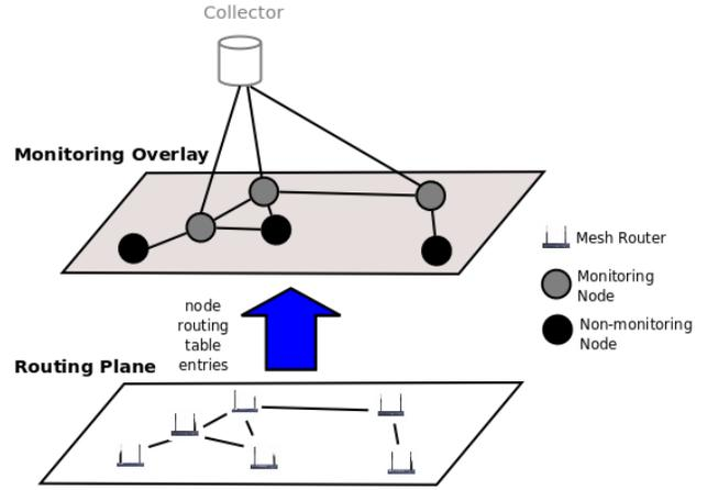
Fig. 1: Wireless Mesh Network flow monitoring architecture
