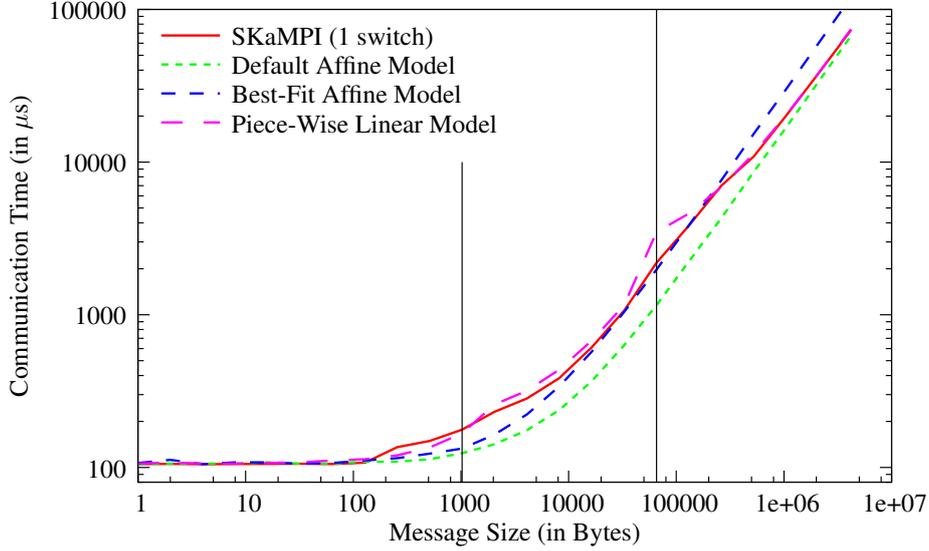
Figure 4: Comparison between a SKaMPI run and SMPI (default affine, best-fit affine and piece-wise linear models) for a ping-pong operation between two machines of the *gdx* cluster using the calibration made on the *griffon* cluster.
