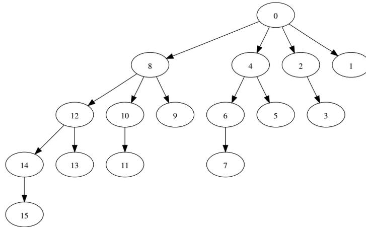
Figure 6: Communication scheme of a binomial tree based `MPI_Scatter` with 16 processes.
