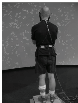
Figure 1. Subject installation in the virtual environment. The subject stands on the force platform in front of the 180° curved full-screen and has to maintain a stabilized balance during the visual flow stimuli.
