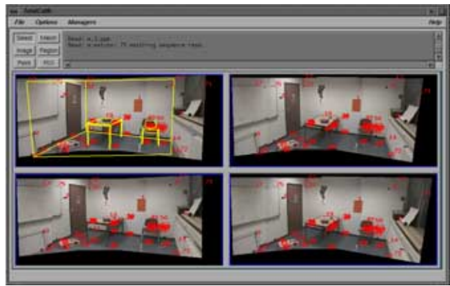
Figure 2: The TotalCalib system to build 3D models of real scenes, using automatic calibration, and epipolar geometry.
