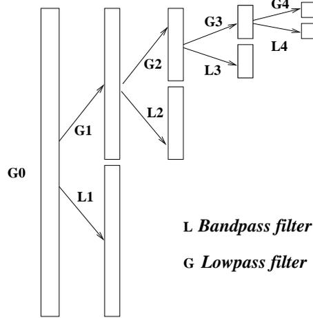
Figure 7: Principle of the multi-resolution filtering process.
