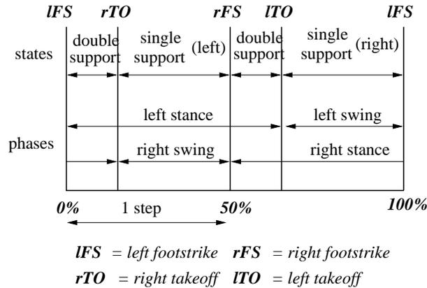
Figure 2: Characteristic phases of a walking motion.
