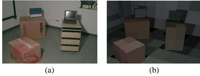
Fig. 4. (a) The original view of the scene and (b) the corresponding radiosity mesh used to simulate indirect light and dynamic updates; note the coarse subdivision.
