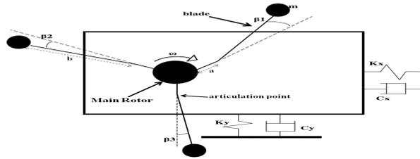
Figure 3: Mechanical model of a helicopter with 3 blades
