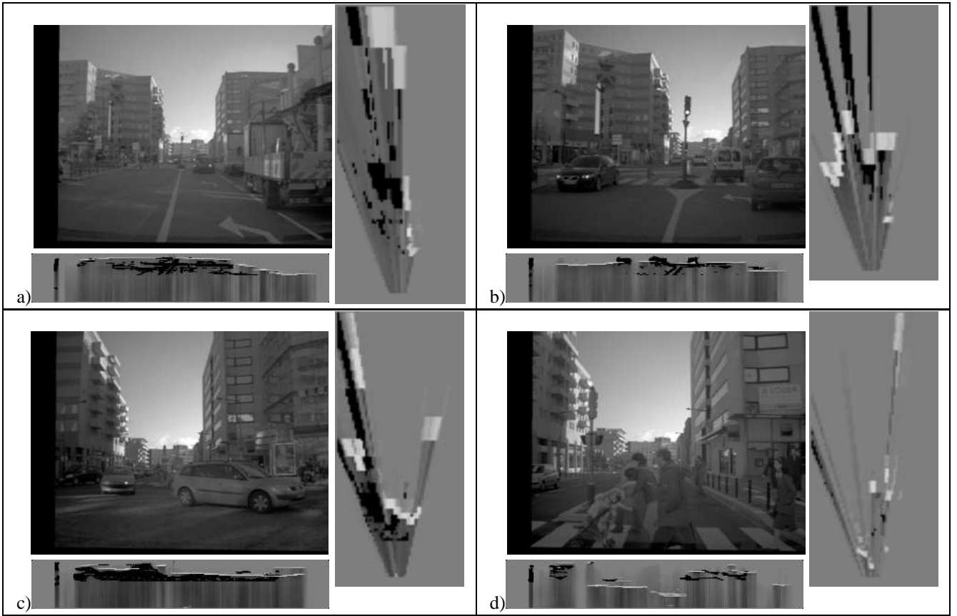
Fig. 4. Typical results obtained with a dataset from the French project LOVe. For each result: the left image of the stereo pair, the occupancy grid in the u -disparity plane and the occupancy grid in Cartesian space.
