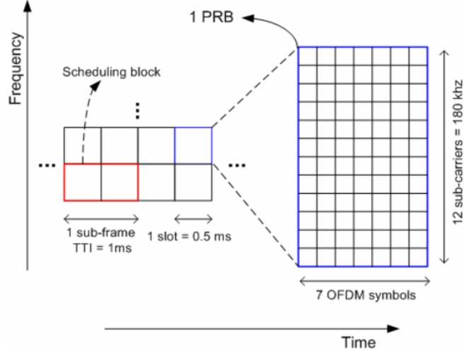
Figure 2: An illustration of resource element in LTE
