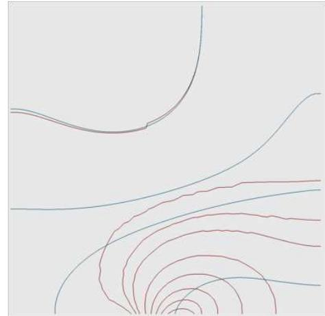
Figure 17: Isolines of the temperature field for a large displacement ( $t = 30s$ ). Blue lines correspond to the simulation, red lines to the fast estimate.
