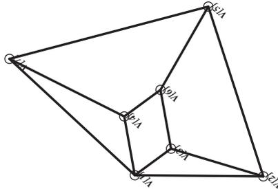
Figure 1: An 11-bar linkage.
