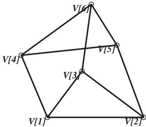
Figure 2: The Desargues linkage or, equivalently, a planar parallel robot.
