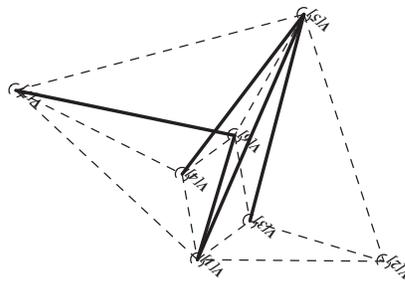
Figure 4: When the edge lengths [15], [16], [35], [45] and [67] are specified as a solution of System (2), the 11-bar linkage has only one assembly mode.
