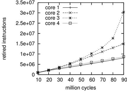
**Figure 4:** Symmetric run of microbenchmark 999 with  $SIZE = 2^{19}$  (Figure 3). Memory bandwidth is 4 bytes/cycle and the L2 replacement policy is a variant of DIP (one PSEL counter per thread). The plot shows the number of retired instructions on each core as a function of time.
