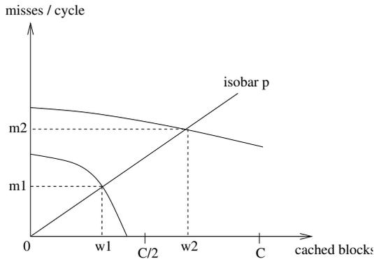
**Figure 2: Example with 2 threads.** The miss rate  $m_i$  of thread  $i$  is assumed to be a function of the number  $w_i$  of cached blocks. The equilibrium partition  $(w_1, w_2)$  is such that the two threads have equal cache pressure  $p = m_1/w_1 = m_2/w_2$ , hence the points  $(w_1, m_1)$  and  $(w_2, m_2)$  lie on the same *isobar* (straight line whose slope is the pressure  $p$ ). The equilibrium partition is obtained by rotating the isobar around the origin till  $w_1 + w_2 = C$ .
