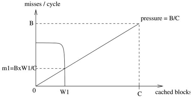
**Figure 8: Cache pressure model.** Cache capacity is  $C$  and bandwidth (maximum number of misses per cycle) is  $B$ . On this example, thread #1 has a working set of size  $W_1$  and a miss rate curve that drops suddenly when  $W_1$  blocks are cached. If the other threads are able to saturate bandwidth, the cache pressure is  $B/C$  and the miss rate  $m_1$  of thread #1 is  $\frac{W_1}{C}B$ . Thus increasing bandwidth increases cache pressure and decreases thread #1 performance.
