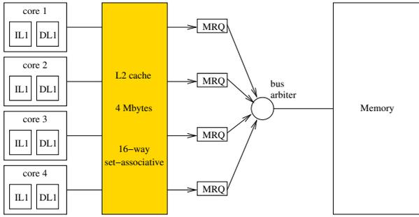
Figure 1: Symmetric multicore simulated in this study.
