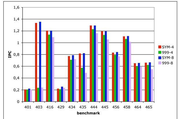
**Figure 7:** IPC for a subset of our benchmarks. The benchmark is run on core #1. Two workloads are considered for the 3 remaining cores : workload SYM runs a copy of the benchmark on each core (symmetric run) and workload 999 runs a copy of microbenchmark 999 on each core. For both workloads, we show the IPC when memory bandwidth is 4 bytes/cycle (SYM-4 and 999-4) and when it is 8 bytes/cycle (SYM-8 and 999-8).
