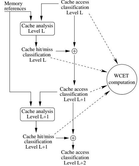
Figure 4: Multi-level non-inclusive data cache analysis framework
