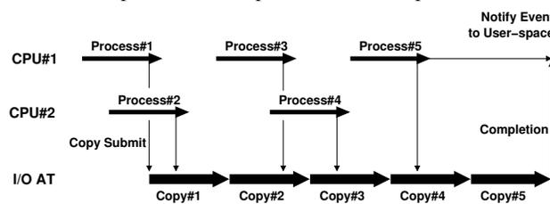
Figure 8: Timeline of the receipt of a 5-packets large message on 2 processors with I/O AT offload of asynchronous copies. The last packet callback waits for the completion of all asynchronous copies before notifying user-space of the receipt completion. All other packet callbacks release the CPU right after processing the packet header (*Process#n*) and submitting the asynchronous copy (*Copy#n*).
