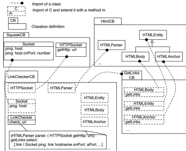
Fig. 2. The dead-link checker modularized with classboxes.
