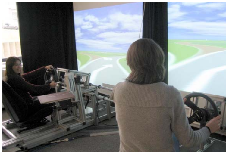
Figure 2: Theatre- technique with driver (left) and confederate (right), mechanically coupled. In contrast to the original Wizard-of-Oz-technique, in the theatre technique the curtain is open, and both driver and confederate play through different use cases and system behaviours.
