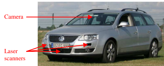
Fig. 3 FASCar demonstrator vehicle
