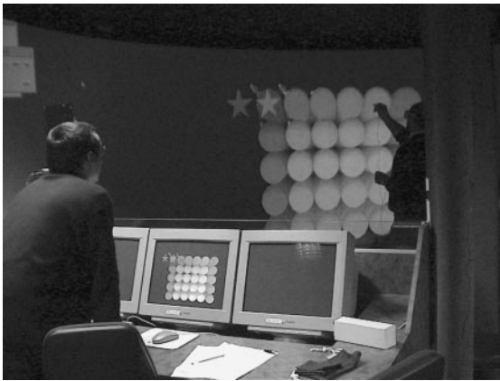
Figure 9: Interaction with 2 LEDs to obtain a 3D mouse : just after the first click to grasp the object
