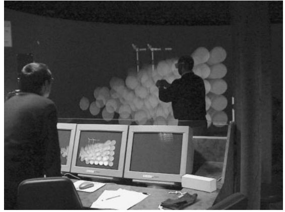
Figure 10: Interaction with 2 LEDs to obtain a 3D mouse : the second click to release the object
